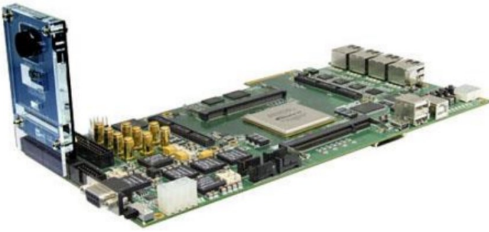
Figure 1-3 Connect the D5M to DE2-115 board's expansion port
