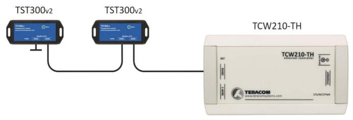
Attention: The last sensor in the chain should have a terminator installed on the free RJ45 socket.
