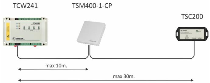
"Star" topology can be used only as a last resort for up to 4 sensors and a total cable length of up to 10 meters.
