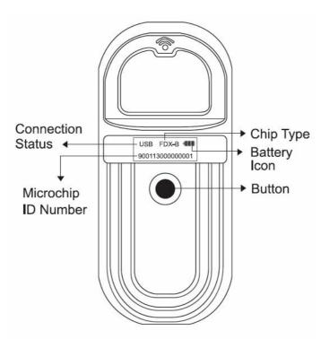
Getting to know the reader. This item is a wireless handheld microchip reader that can read ISO FDX-B coded radio frequency identification tags. It has very simple controls and a high-brightness OLED display which allows you to read the numbers even in bright sunlight. With built-in memory, it is able to store up to 128 ID tag codes, which can be downloaded to a computer via a USB cable connection. Optimum performance ensures that it is a perfect deal for animal traceability and management.
