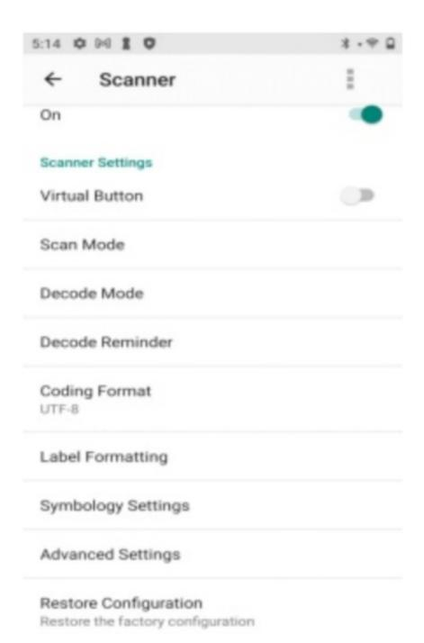
By default, the integrated scan engine is enabled for scanning. It supports omni-directional barcode scanning, and an aiming beam is provided to help assist with targeting barcodes.
