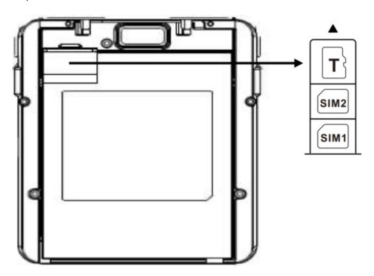
Note: Always power off the terminal before attempting to install or remove a card.
