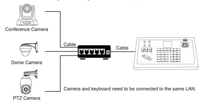
Connect the camera and joystick controller in the same LAN and ensure their IP address in the same network segment, such as 192.168.1.123 and 192.168.1.111 belong to the same network segment, while 192.168.1.123
