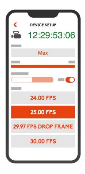
Pressing briefly on a Tentacle in the monitoring screen, will start a connection to this device and allows you to set timecode, frame rate, user bits and more. The general parameters are the same across all setup apps for the different operating systems.
