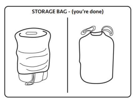
It is important that you work the bag down to the top of the roll—flip the unit and pull the bag up over the top of the inflatable amusement device
