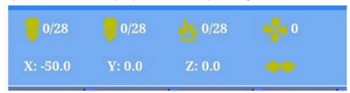
5. ) **Control interface:** Some basic operations can be performed, such as moving the position of each axis, switching nozzles, and returning to zero for each axis
