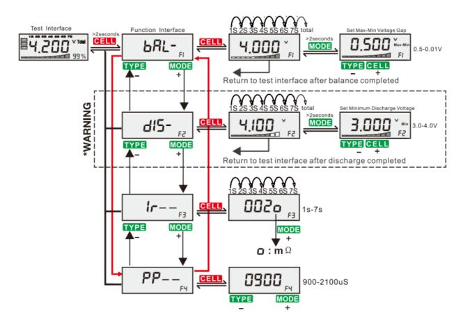
**WARNING:** To avoid overheating, the discharge function can only be used for less than 6 mins each time. After that, please let the unit cool down to room temperature before discharging again. DO NOT leave your battery discharging with this device unattended.
