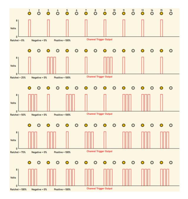
It needs to be noted that ratcheting can only affect steps that the user has assigned as "active" ie. the LED needs to be illuminated for a step to ratchet. Even if an inactive step is triggered via negative probability, these steps will never ratchet.
