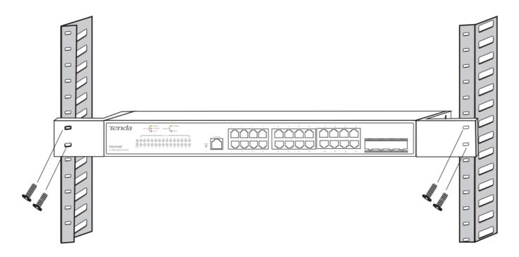
Step 3 Mount the switch at a proper height on the subrack and fix it to the rack with screws (self-prepared).
