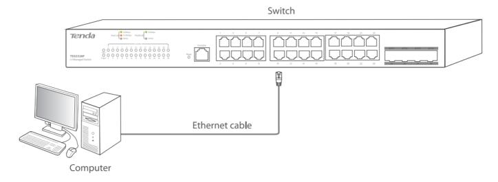
**Step 2** Set the IP address of the computer to an unused one in the same network segment as the switch. For example, the default IP address of the switch is 192.168.0.1, set the IP address of the computer to 192.168.0.X (X ranges from 2 to 254 and is not occupied) and subnet mask to 255.255.255.0.
