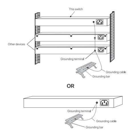
**Note:** Connect the grounding cable to the grounding system in the equipment room. Do NOT connect it toa fire hose or lightning rod.
