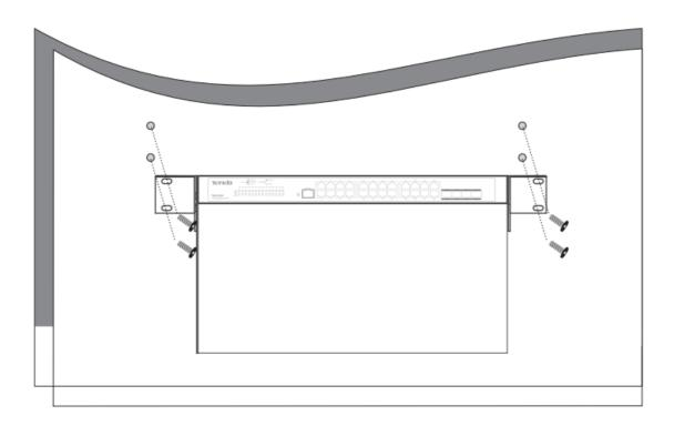
**Note:** Do NOT install the switch with its ventilation openings facing downward, otherwise there will be potential safety hazards.
