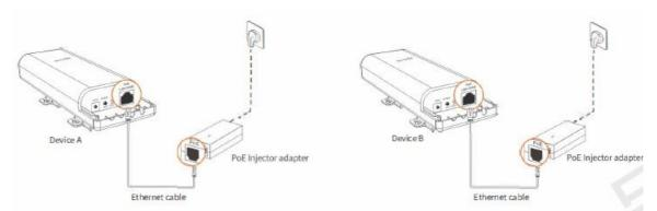
2. Please switch the mode button(STA/OFF/AP) of device A to AP position, then press and hold the Bridge/RST button for 3-7s (it is suggested to count from 1 to 5), then release it. The signal strength LED (LEDI, LED2, LED3) on the rear panel will start to blink.
