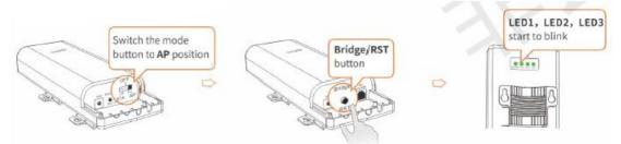
3. When the LED of Device A is blinking, within 2 minutes, please switch the mode button (STA/OFF/AP) of Device B to STA position, then press and hold the Bridge/RST button of device B for 3-7 seconds, then release it. The signal strength LED (LEDI, LED2, LED3) on the rear panel will start to blink. Two devices will start to negotiate to bridge together.
