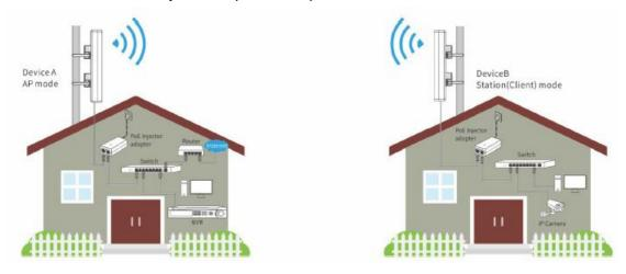
Within 2km visual range, it is capable to do 30pcs 720P (Impx) CCTV Surveillance. Within 5km visual range, it is capable to dol0pcs 720P (Impx) CCTV Surveillance.
