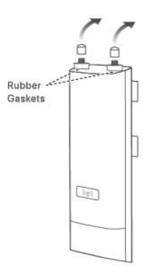
2. Connect the antennas to the SMA connectors.
