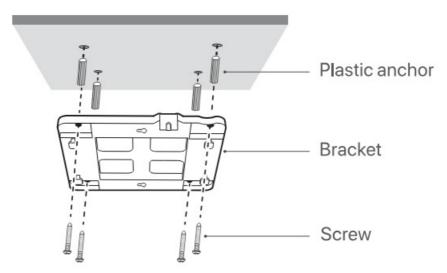
• Option B: Insert the included screws into the screw holes on the bracket and fix them into the included plastic nuts using a screwdriver.
