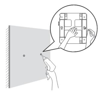
3. Knock the included plastic anchors into the holes using a rubber hammer. Then use a screwdriver to fix the included screws into the plastic anchors. The distance between the inside surface of the screw header and the edge of the plastic anchor should not be less than 2.5 mm, to make sure that the AP can be hung on the screws firmly.
