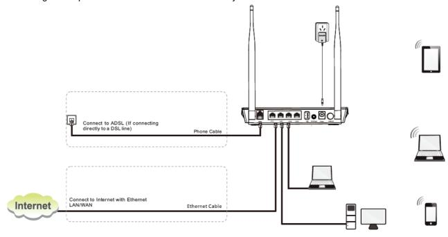
This quick install guide applies to the following four models: D301, D302, D152 and D151. The D301 is used as an example here.
