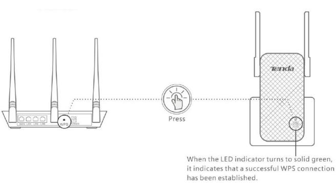
3. Relocate the extender to other electrical outlet. Observe the LED indicator on the extender to choose an optimum extended location for best WiFi performance.
