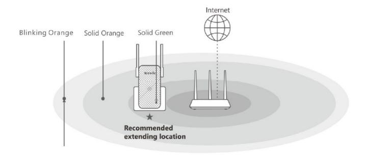
Keep moving the extender to outlets closer to the router until the LED indicator on the extender lights solid green.
