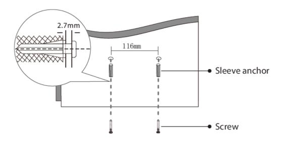
Step 2: Align the slots of the switch to the screw heads, and slip the switch to make it fixed on the screws firmly.
