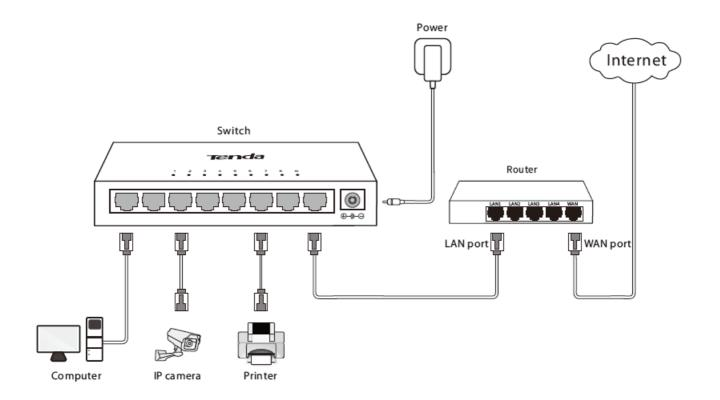
**Tip:**All ports of your switch support the auto MDI/MDIX function, indicating that either straight cable or crossover cable is acceptable to connect your switch to Ethernet devices.
