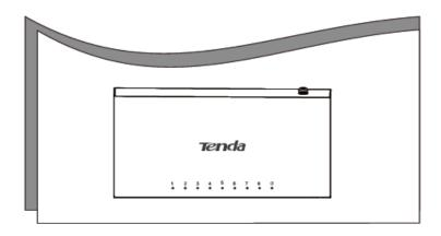
Note: For safety, do not face the air vents of the switch down
