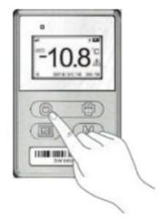
Long press the "Start/Stop" button till "REC" has been showing on the LCD interface, the device is ready to monitor. At the same time, the record quantity also will be shown on the LCD interface
