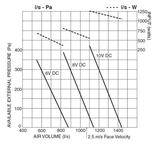
Note: Airflows are for a dry coil. Reduce airflow by 10% in high moisture removal conditions. In a free blow or low resistance application, beware of exceeding indoor fan motor's full load amp limit (refer Specification page). As filters are optional, the fan air flows given are for units installed without filters. VPA 160RKTG-P
