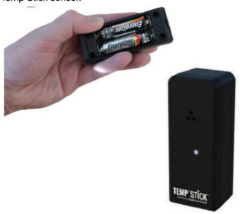
The LED light on your Temp Stick will start blinking indicating it is in Setup Mode.
