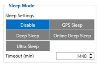
When in GPS sleep mode, TFT100 turns the GPS module off and continues making new periodic records. As a result power usage decreases, in turn saving vehicle battery.
