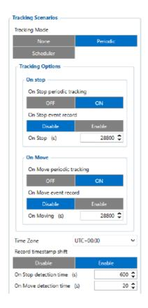
On Stop periodic tracking – enable or disable periodic data sending when device is On Stop. Device will generate and send normal record with event ID 0 and movement AVL ID 240 with a value of 0.
