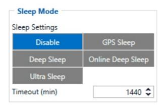
Please note that power saving depends on two configurable parameters: Send Period and Minimum Record Saving Period in "X on Stop Mode". When records are sent successfully in deep sleep mode, open link timeout counter will be skipped and MTB100 will enter deep sleep mode immediately.
