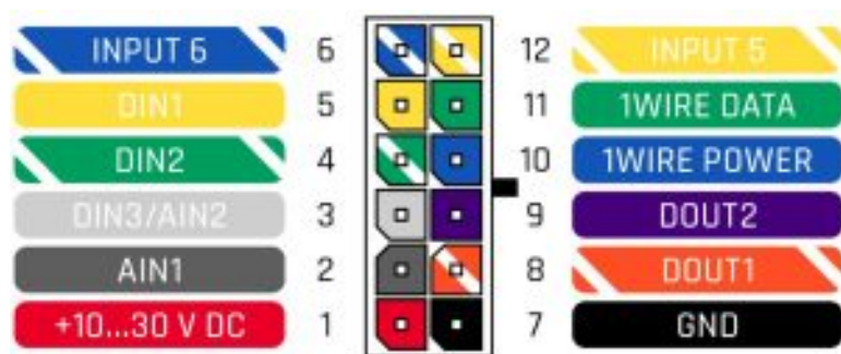
Figure 2 FMB120 2×6 socket pinout
