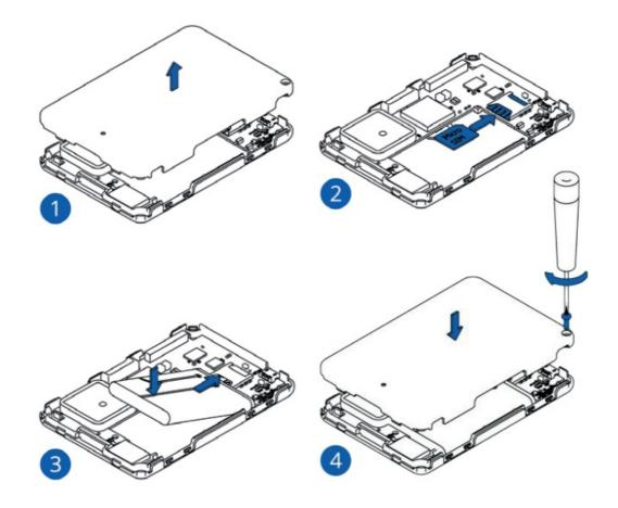
Micro-SIM card insertion/removal must be performed when device is turned off. Otherwise Micro-SIM card might be damaged or device will not detect it.
