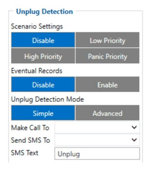
An event will be generated when FMC13A is unplugged from external power or plugged back in again.
