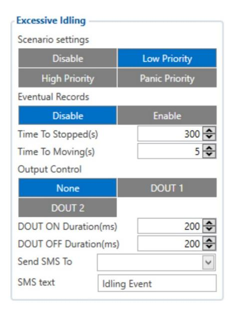
When vehicle stops for a specific amount of time the scenario is activated, a record will be generated and digital output status will be changed to 1 when configured. You can configure the time it takes to turn on this scenario (Time to Stopped). Scenario is activated until the vehicle starts moving(movement is detected only by the accelerometer) and keeps moving for an amount of time that is configured. You can configure the time it takes to turn off this scenario (Time to Moving) info
