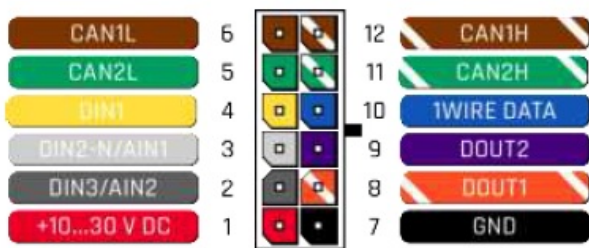
Figure 2 FMB140 2x6 socket pinout
