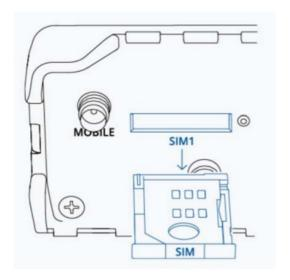
Slide the SIM holder back into the router .
