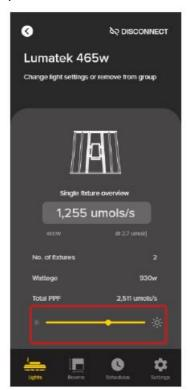
3. Alternatively, enter the desired PPF setting directly in the input box.
