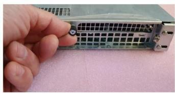
3. Pull the top cover plate from the knob screw, and lift the top cover in order to remove it.
