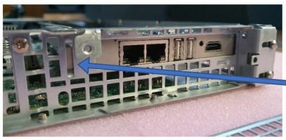
The tip of the card's bracket slides in this slot
