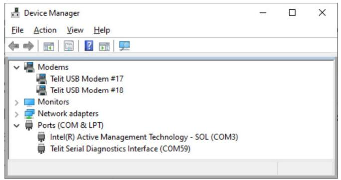
USB Modem ports are ACM devices and can be used as AT Command interface. To identify the corresponding COM port number, just right click on one of the two Telit USB Modem entries, select Properties, then Modem tab. The picture shows the Telit USB Modem properties. In this example Windows 10 system binds USB #17 with
