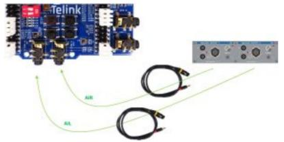
• All jumpers are kept in the default setting, and the connection of the audio output path is as below. Some audio analyzers can be used for testing, such as APx525.
