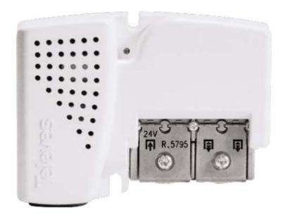
Domestic 24 V power supply (130 mA) that powers equipment through the input coaxial cable while allowing the transmission of the TV signal. Included in the installation is power to either the mast amplifiers or a BOSS system. Furthermore, it is equipped with two outputs.
