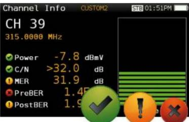
Easy decision-making Reduce installation mistakes with the on-screen Pass/Fail indicators, a graphical tool that helps and speeds up the interpretation of measurement results. Different thresholds are available depending on the network area to be analyzed: headend, multi-band amplifiers, bridging connection, connection records, user home, etc. Besides the pre-set values, you will be able to customize your own threshold values.
