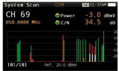
Monitored installation Scan each existing analogue and digital channel in real time to determine the overall system frequency response. This function leverages the location-based thresholds to clearly show whether the signal levels meet the cable systems' specifications with green, yellow and red bars. This feature provides an easy-to-understand, real-time view of the system, including the BER and MER values of the selected channel.
