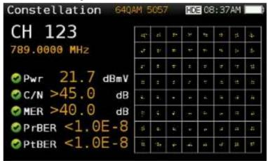
Fine-tune your digitals Constellation analysis is essential for determining the quality of digital signals. Constellation diagrams help detecting noise, jitter, interference and signal saturation, and all the variables that could impact signal quality, eventually leading to service suspension. By visually inspecting the size and shape of the dots in the constellation matrix, the technician will be able to easily identify the nature of the problem
