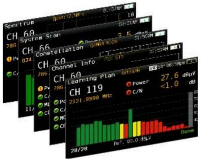
Pass/Fail indicators A full range of functionalities such as Single-channel measurements, Constellation diagram, Spectrum analyser, Service identification, Data logs, Channel plan auto-learning, and more.
