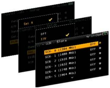
signal from any satellite H30FLEX allows you to configure the parameters required for the reception of your satellite signal. To do this, H30FLEX allows preamplifier powering, and configuration of both DiSEqC and SCR parameters.
