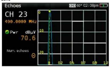
Optimal signal reception In terms of terrestrial signal reception, controlling the absence of any echoes that could jeopardize reception is crucial. H30FLEX displays the echoes of the received signal, allowing the installer to minimize them for optimal signal reception.
