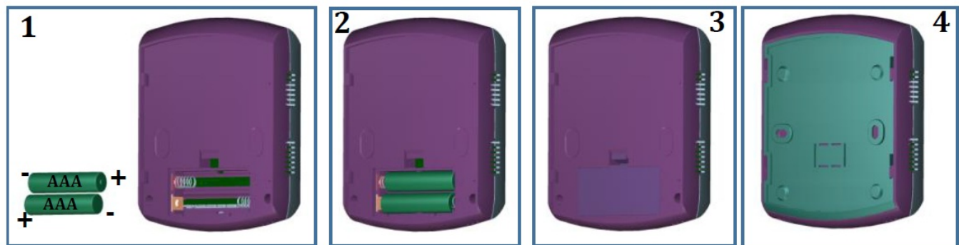
Figure 10. . Steps for inserting batteries and then assembling the device
