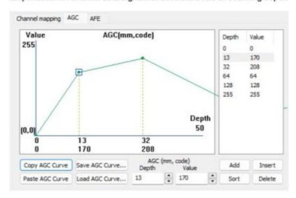
AGC control affects both B-mode images and channel RF data. The points can be created interactively by the left mouse click on the chart at the desired location and deleted by the right mouse click nearby point to delete. The points could be added by using edit fields (Depth, Value) and confirming by button Add (Insert button creates blank value). There is a possibility to Sort AGC points and Delete some points, to Copy, Paste, Save, and Load the AGC curve.
