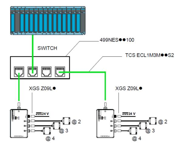
For further information on station configuration and wiring, see the Ositrack Compact Station Guide DIA4ED3051001. The splitter box contains a line terminator.
