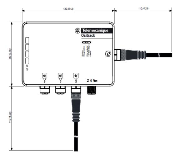
M12 connector maximum tightening torque = 10 Nm (88.5 lbf.in)
