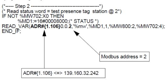
During programming, use the XWAY address to specify the station. The Modbus address is set to 2.
