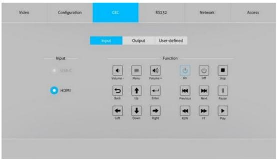
Click to send the corresponding CEC command to the device connected to either the transmitter or receiver's HDMI output.
