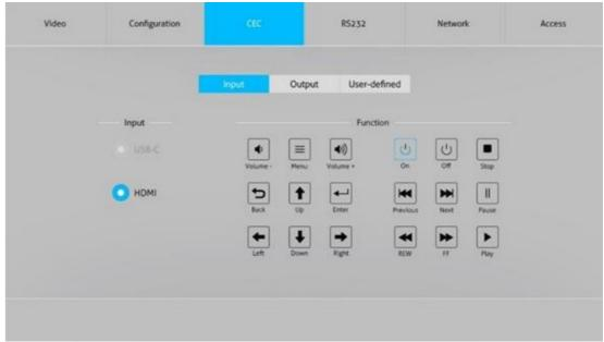
Click to send the corresponding CEC command to the device connected to the HDMI input
