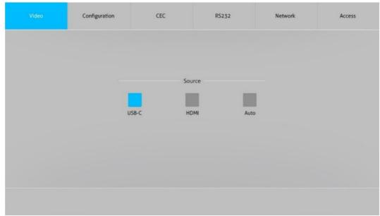
Select HDMI or USB-C as the active video input source, or toggle Auto-Switching mode **5.2 Configuration Tab**
