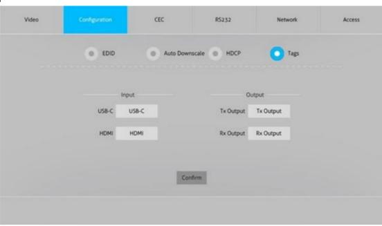
Customize the tags for the HDMI and USB-C inputs, and for the transmitter and receiver HDMI outputs
