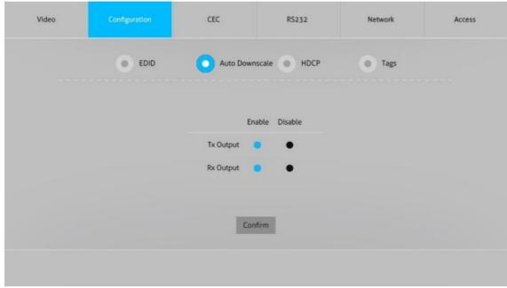
Enable or disable automatic down-scaling for the transmitter and receiver video outputs **5.2.3 HDCP**
