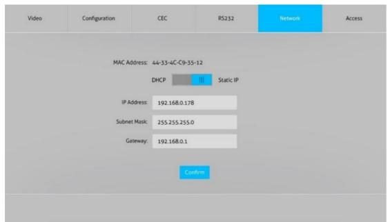
Choose whether the switcher is set to a Static IP address or gets a DHCP automatically from the network DHCP server.
