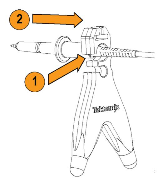
Position the base of the probe holder on your circuit where it can maintain stability while contacting the test point.
