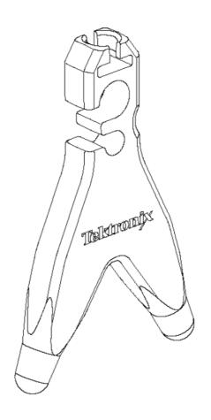
The weight of the probe holder keeps the probe in contact with your circuit, and the non-skid base keeps the
