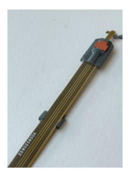
4. Adhesive tape can be placed on the IC package top. Glue can be applied onto the tape under one or both wings. This allows you to later easily remove the tip from the DUT by removing the tape.
