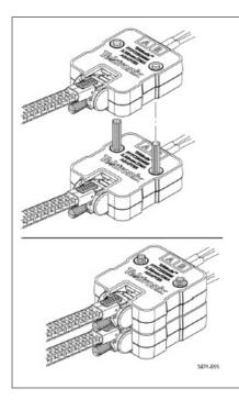
Use two gray adapters to stack two P77C292 MM adapters; use two black adapters to stack three or four P77C292MM adapters.
