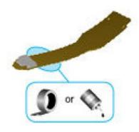
3. The flexible holding tabs (sides) of the clip provide strain relief. This allows you to secure the clip to the long body of the tip. You can use a liquid adhesive beneath the clip to secure the tip to the DUT.
