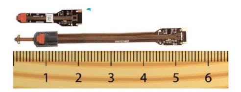
The tip wings can be used to place adhesive on or they can be trimmed if required for placement.
