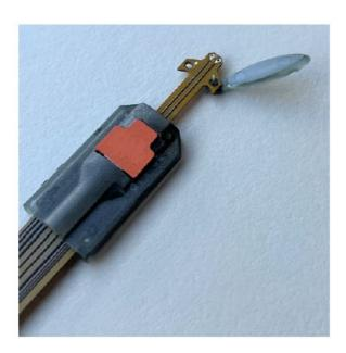
2. Use liquid adhesive to secure the handle as needed. If you do not need the handle, remove it once you have placed the tip. (See emiuv.com for adhesives.)
