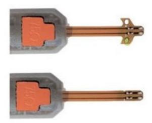
You can visually identify the FLR A versus B tips. The A versions have a blue plastic housing. In addition, there is an intentional cutout on the A tips near the plastic housing that is not present on the B tips.
