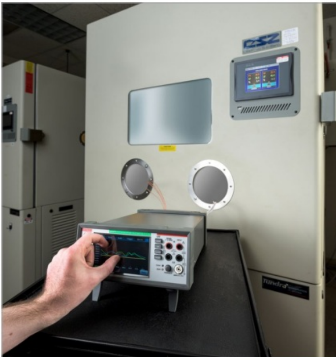
Figure 2: A Tektronix DAQ6510 monitoring components inside an environmental test chamber.
