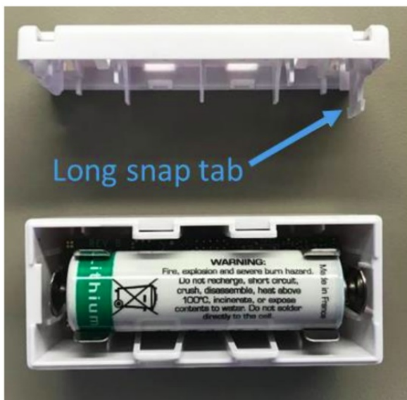
Figure 2-5: Proper Replacement Orientation of the Battery Cover
