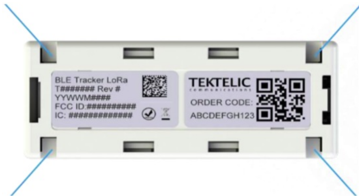
Figure 2-2: The Mounting Hole Locations on the Bottom of the Tracker
