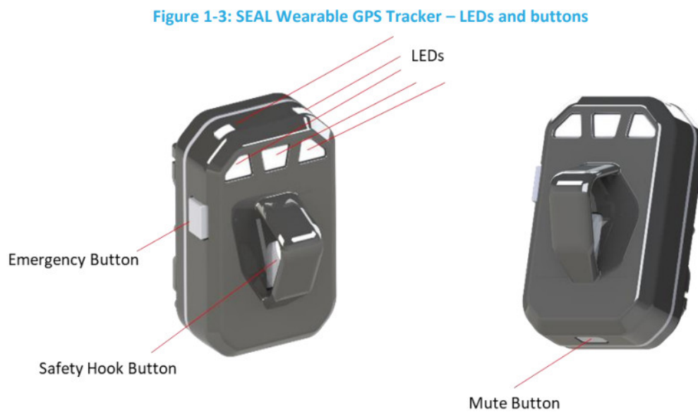
Figure 1-3: SEAL Wearable GPS Tracker – LEDs and buttons
