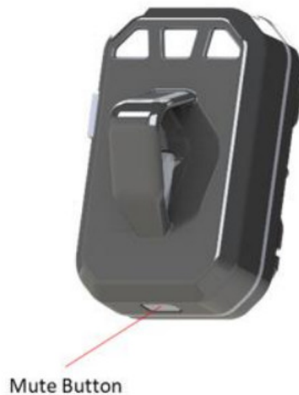
Figure 2-1: SEAL/SEAL-Ex with clip showing the mute button.
