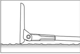
To minimize interference while probing the ground, lay the metal detector down with the searchcoil perpendicular to the ground.
