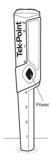
As a result of the Tek-Point's extreme sensitivity, you may encounter ground mineralization conditions that require an alternate calibration method. If the pinpointer "falses", or beeps erratically, when touched to the ground you may want to turn it on after touching it to the ground.
