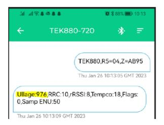
If the ullage value is not correct; then please review the installation and mounting of the sensor to ensure there are no obstructions and that the sensor is mounted horizontally.
