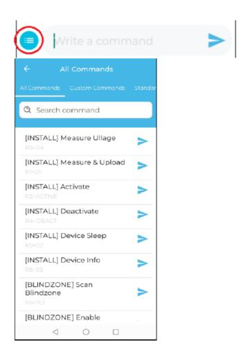
b) Select the correct liquid type and setup to be measured. The sensor uses a series of internal settings /coefficients that optimise its performance for different liquid types. In the example shown below the installer can select "Hydrocarbon – Oil Setup" from the command list to indicate to the sensor that these internal coefficients should be used.
