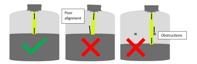
Once the sensor is mounted, it is important to carefully measure the usable tank height. This is because the radar sensor needs to know the overall scanning distance to protect the battery and prevent any erroneous reflections from pooling water from being generated.
