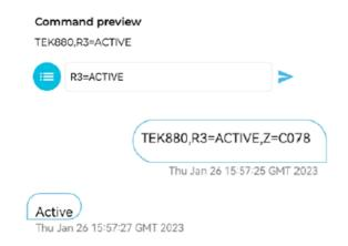
Once this command is complete, then the unit is installed and is correctly communicating with the server and will return to sleep until the next scheduled dial-in.
