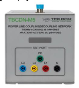
The TBCDN-M5 is compliant with IEC 61000-4-6 Annex D2. It is designed to inject common mode disturbance signals in the frequency range from 150 kHz to 230 MHz into unscreened AC and DC power supply lines.
