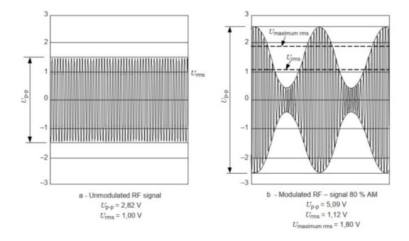
Consequently, the level of the modulated signal must be 5.1 dB higher than the test levels specified by the standard. Adding a 6dB attenuator to improve the matching of the RF power amplifiers would require the following amplifier output power:
