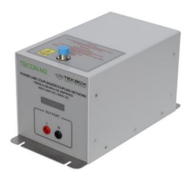
The TBCDN-M2 is a Coupling Decoupling Network for conducted immunity testing according to IEC 61000-4-6. The TBCDN-M2 is compliant with IEC 61000-4-6 Annex D2. It is designed to inject common mode disturbance signals in the frequency range from 150 kHz to 230 MHz into unscreened AC and DC power supply lines.
