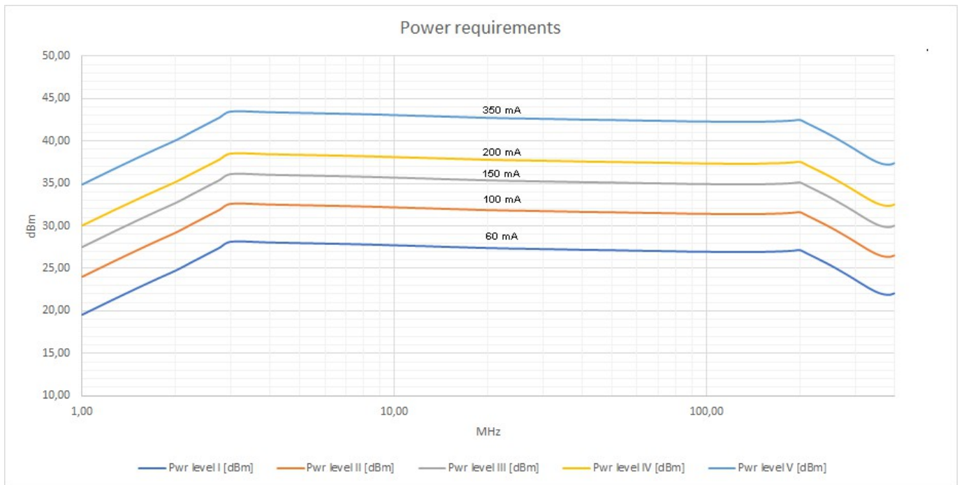
Figure 4: corresponding required RMS forward power into the TBBCI1-800K420 BCI probe
